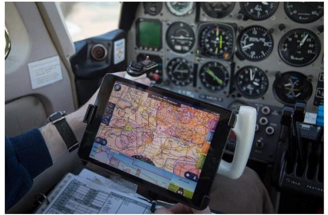
A yoke-mount gives a good view of the device, but you may get glare and it can block controls.
