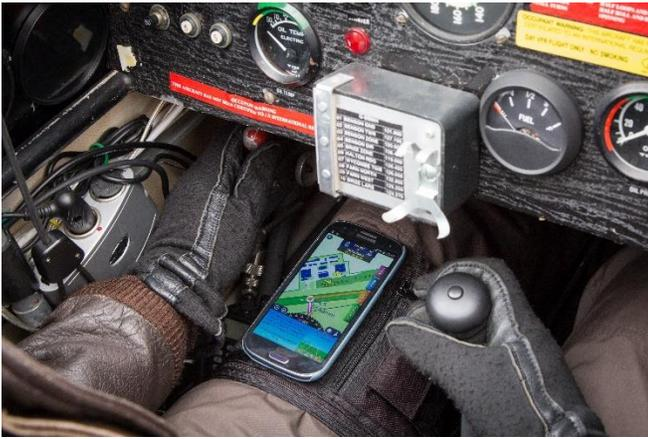
A leg-mount allows the unit to be shaded, is close enough to read and is ideal for a small cockpit.
