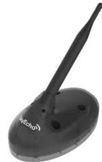
According to CAP 1391, Electronic Conspicuity devices capable of 1090MHz extended squitter do not require specific approval by the National IFF/SSR Committee (NISC) to operate, providing they comply with the requirements of Annex 10 to the Convention on International Civil Aviation Volume IV, or Standardisation Agreement (STANAG) 4193, as appropriate. The Sky Echo unit is CAP1391 approved.
